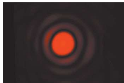
Figure 36-10 The diffraction pattern of a circular aperture. Note the central maximum and the circular secondary maxima. The figure has been overexposed to bring out these secondary maxima, which are much less intense than the central maximum.
